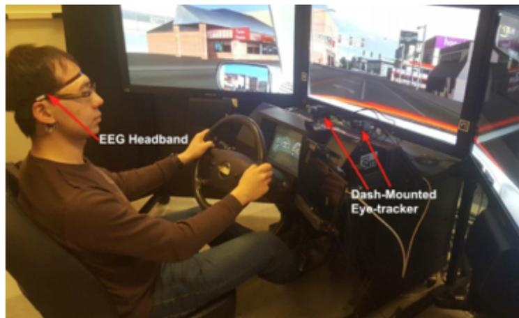
Figure 2: NADS Driving Simulator and placement of eye-tracker.
