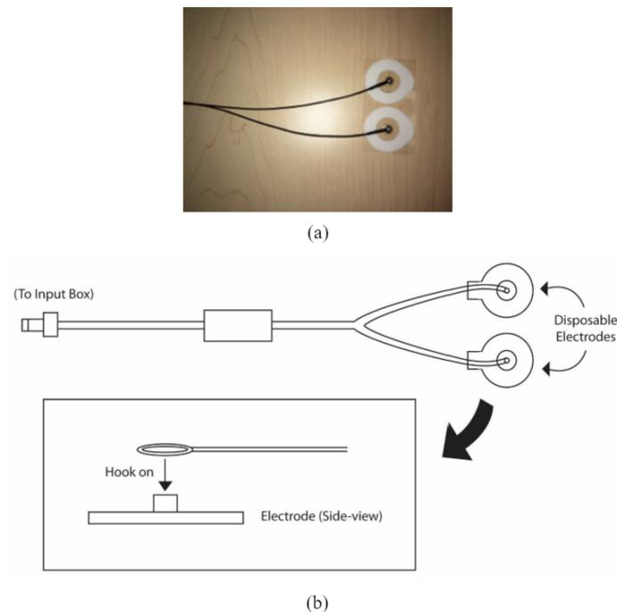
Figure 7: GSR device (a), and wiring setup (b).
