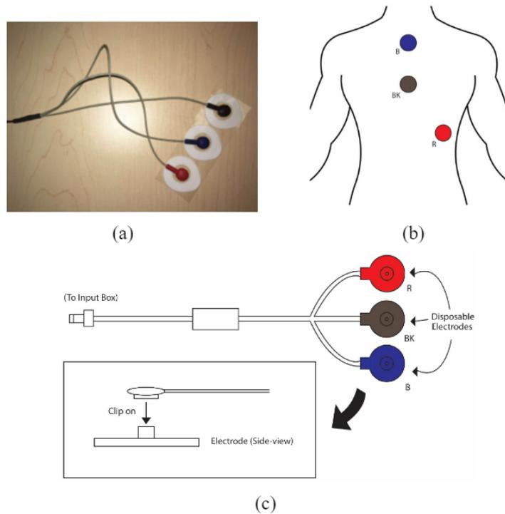
Figure 5: ECG device (a), placement (b), and wiring setup (c).
