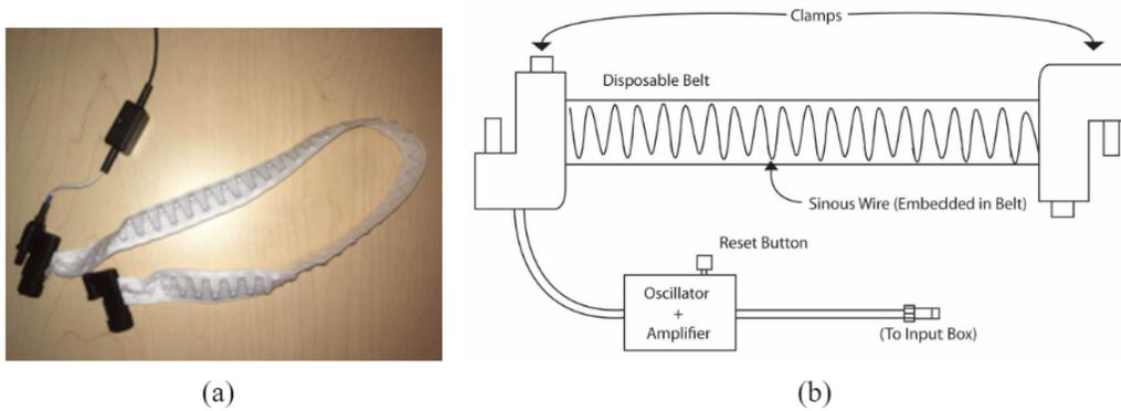
Figure 6: RESP device (a), and wiring setup (b).
