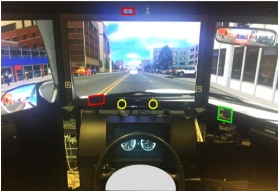
Figure 3: Camera and eye-tracker placements in the driving simulator. The webcams (left and upper) are framed in red, while GoPro camera (right) is framed in green. Eye-tracker cameras (centre) are also marked (in yellow). The grey area at lower middle of the image represents the approximate location of participant's head.
