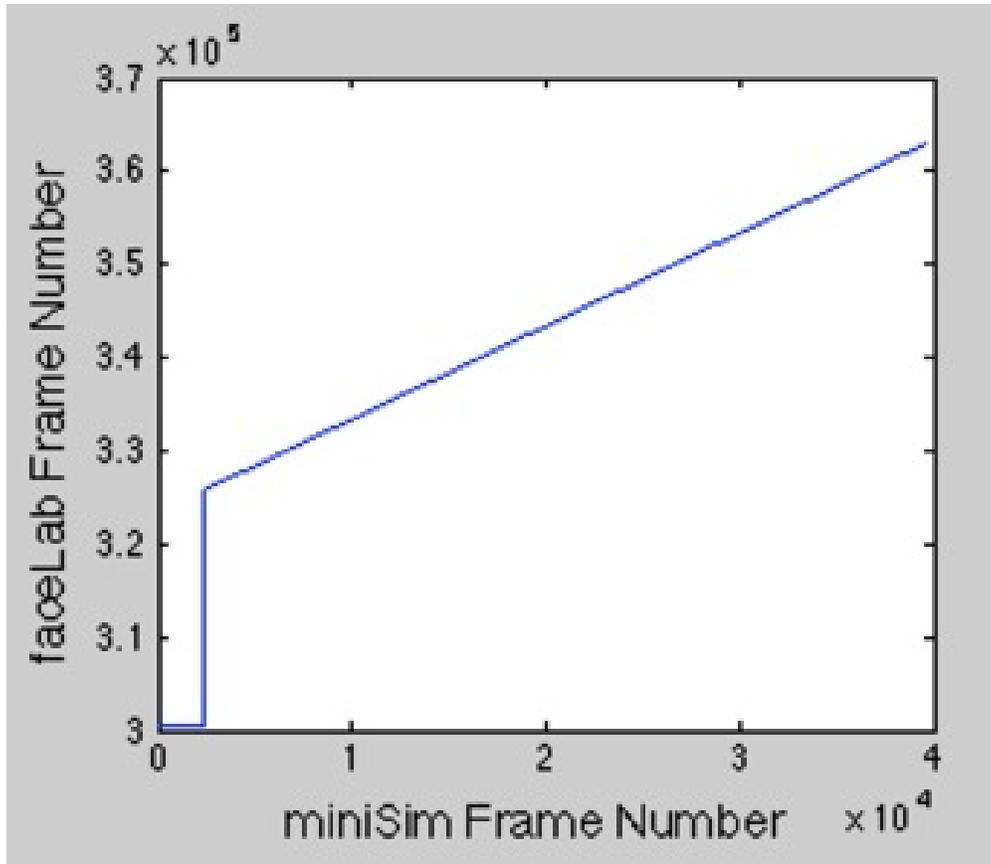
Figure 11: Example of the FaceLab frame number that was received by miniSim (this is the data of Participant 7’s 2-back drive). Notice how the FaceLab frame number takes a jump near the beginning of the recording; it then becomes stabilized and increases steadily.
