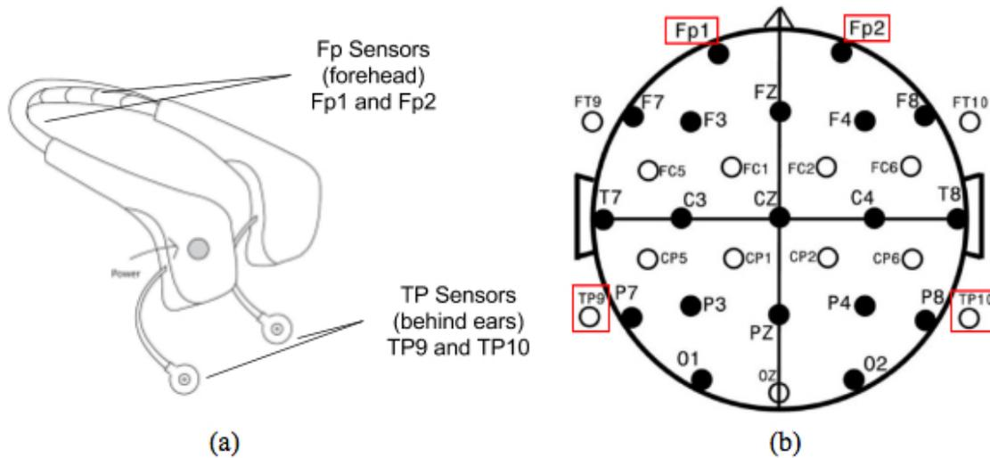
Figure 10: EEG data collection positions. To see how it is worn on a participant, refer to Figure 2. (a) The Muse EEG headband. (b) EEG positions. The red rectangles highlight the positions used in this experiment.
