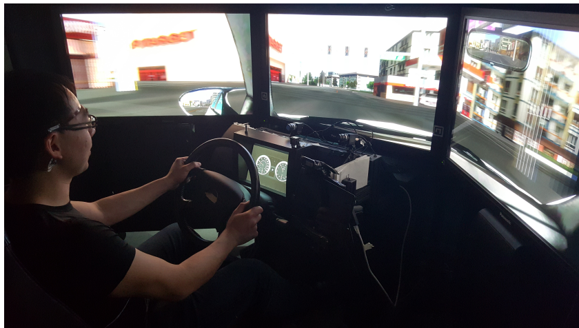
Figure 3.2: The NADS miniSim Driving Simulator displays mid-fidelity rendering of the simulated driving environment on three screens, and the speedometer on another smaller display behind the steering wheel. Other light sources are blocked or turned off to create a more immersing driving environment.
