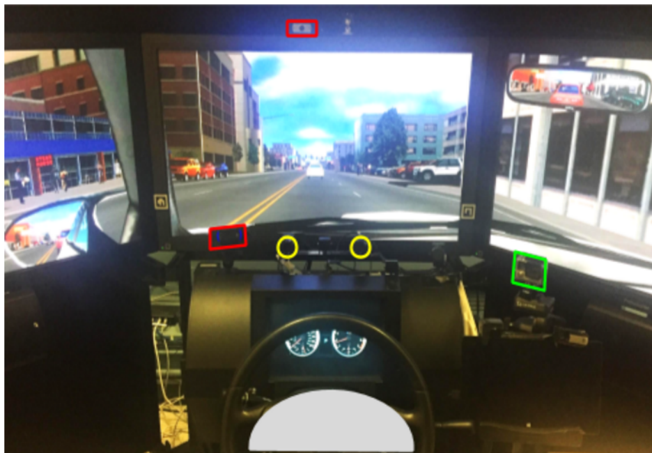
Figure 3.3: Camera and eye-tracker placements in the driving simulator. The webcams (left and upper) are framed in red, while GoPro camera (right) is framed in green. Eye-tracker cameras (centre) are also marked (in yellow). The grey area at lower middle of the image represents the approximate location of participant's head.
